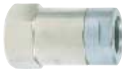
Chuck locks on valve when cocked on threads. Has greater air flow and seat cannot be blown out if seal fails. Has \frac{1}{4} " NPT female thread.
