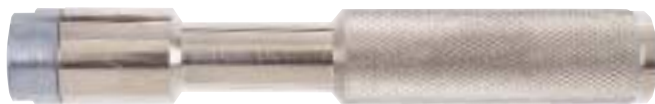
Chuck locks on valve when cocked on threads. Has greater air flow and seat cannot be blown out if seal fails. Has \frac{1}{4} " NPT female thread.
