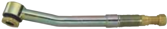
N-1538B 7 7/8" long super large bore turret valve with 15° bend, used on Caterpillar applications.
