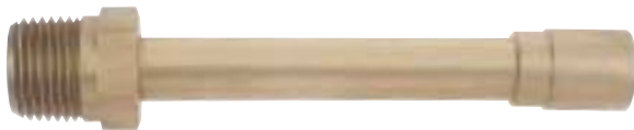
326 Screw-On Air Chuck Has .485-26 internal thread and \frac{1}{2} " NPT external thread. Full flow for seating of tire beads.
